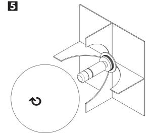
GB Connect the fitting and a connector block / junction box to the mains cables as shown in illustration and wiring diagram. Cover cables connected to the connector block with 2 layers of insulation tape.
