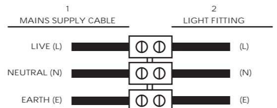
GB Connect the fitting and a connector block / junction box to the mains cables as shown in illustration and wiring diagram. Cover cables connected to the connector block with 2 layers of insulation tape.
